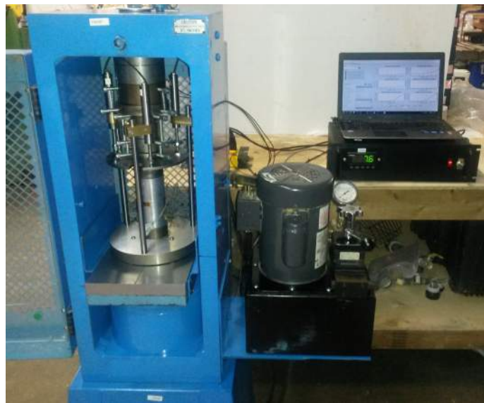
Figure 1: Forney loading frame setup for UCS testing.
